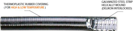
Thermoplastic Rubber Covered Liquid Tight Conduit
